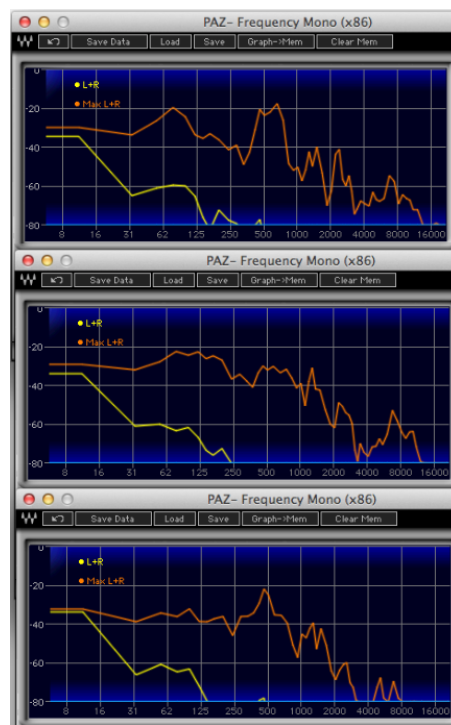
Figure 5.12: Spectrum of same scratching on three parts of the surface
