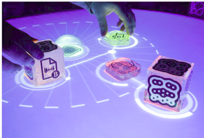
Figure 4.19: Extrinsic Symbols of a reacTable Interface are those digital representations incorporated to the physical artifact.
